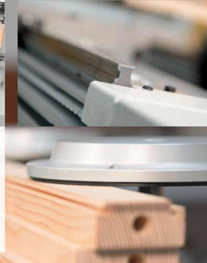
"Jet Fast" automatic positioning by NC. Quick positioning of the panel supports, suction cups and clamps. No intervention by the operator, max. precision and high flexibility.
