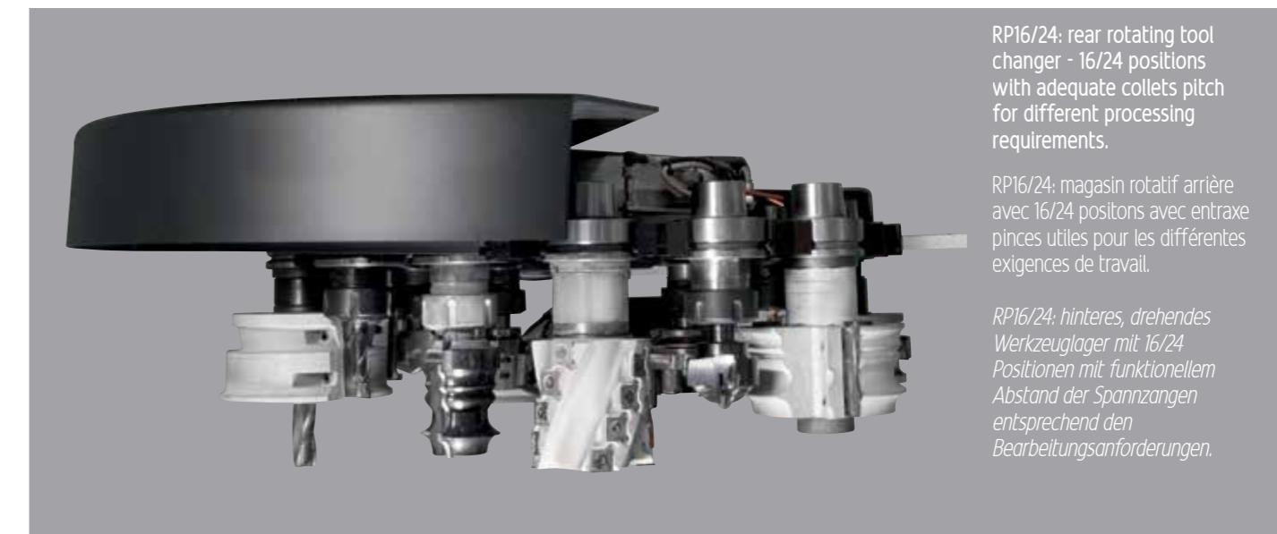
RP16/24: rear rotating tool changer - 16/24 positions with adequate collets pitch for different processing requirements.
