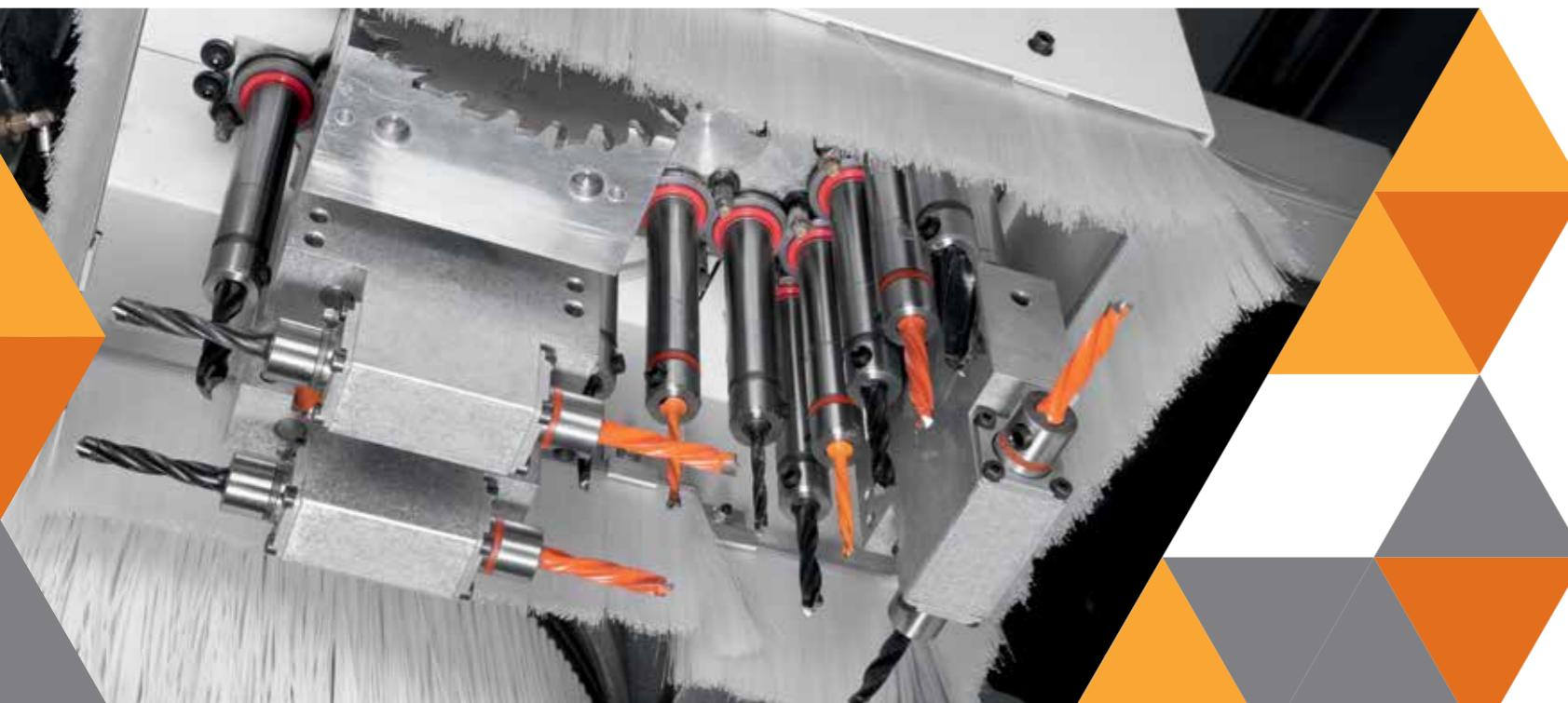
Wide range of tool changers for max. flexibility of processing and quick set up of the working table.
